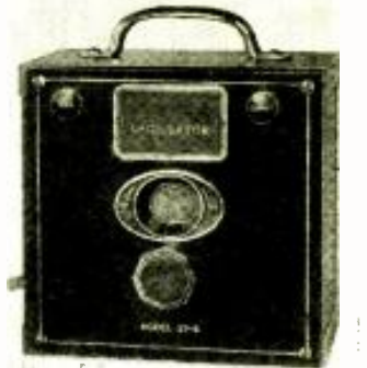
A dual-range service oscillator. (614)
