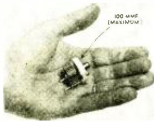
Pee-wee variable condenser. This condenser will fit inside a tube base. (604)
